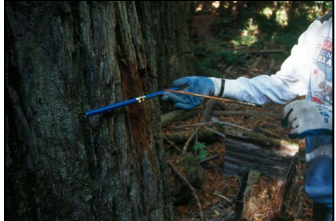
Collecting an increment core (tree ring) sample from a riparian coast redwood tree
